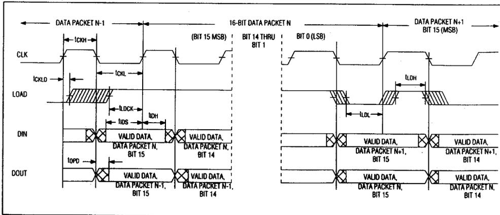
Figure 1. Timing Diagram
